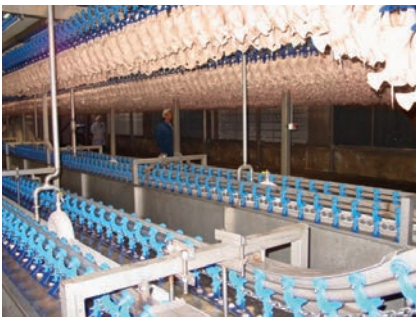
Upper Left: chickens going into the water section of a combi-chiller Lower Left: general combi chiller view Opposite Page: stuffed croquettes
