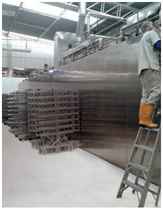
Above: sausage buggies inside the oven Left: semi continuous high capacity cooking, smoking and chilling oven
